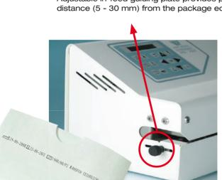
Daily validation with the Seal Check function: temperature, pressure and sealing time can be printed and recorded.
